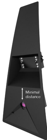
Figure 5: Separation of emitter and receiver (minimum distance)
