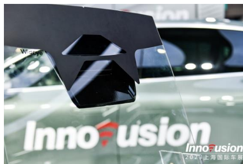
Caption: Built-In Windshield LiDAR / Prototype by Innovusion and Wideye by AGC
